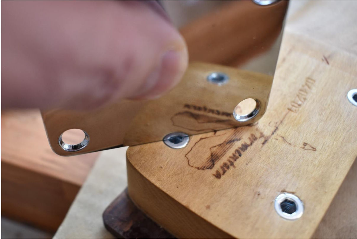
Check that the inserts are flush with the surface!
