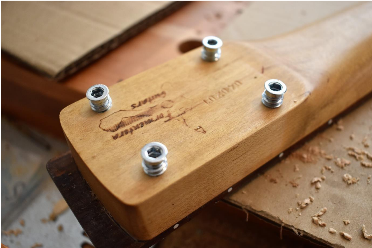
Now the screw inserts are mounted...
