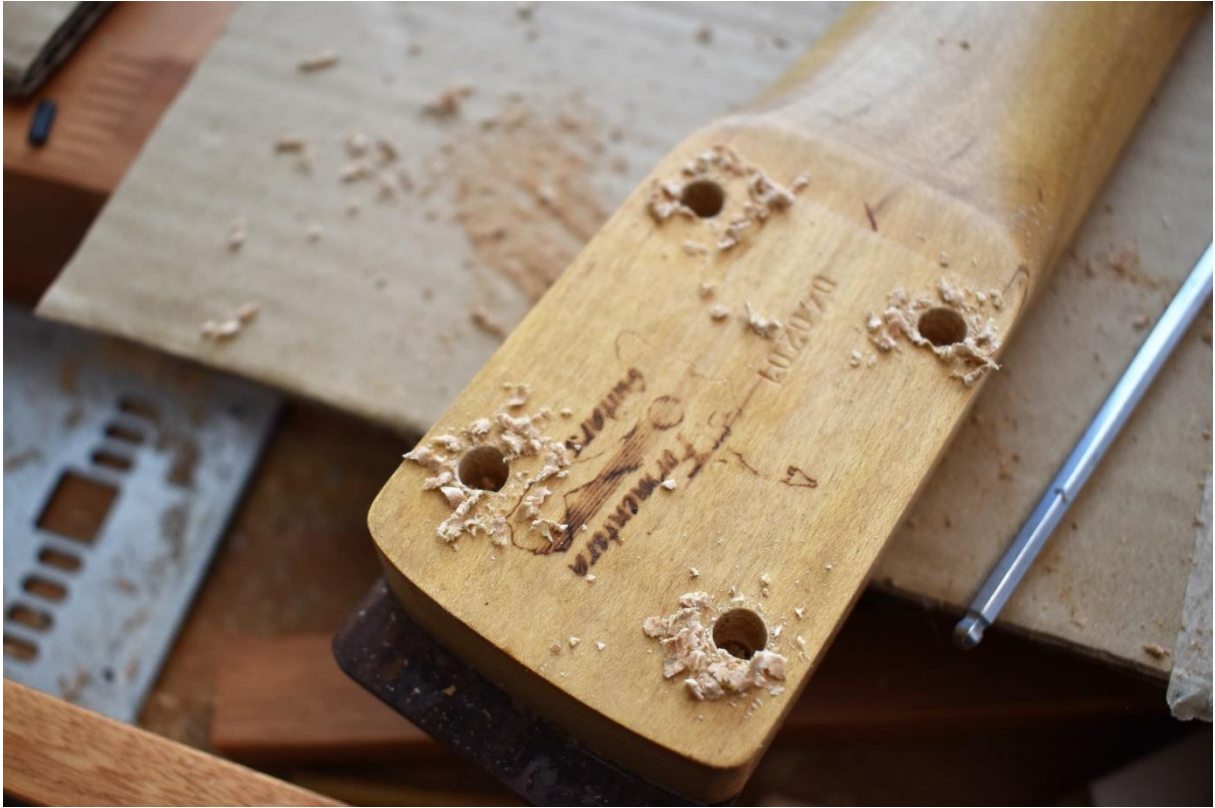
Done, all 4 holes are drilled. Now remove the dust...
